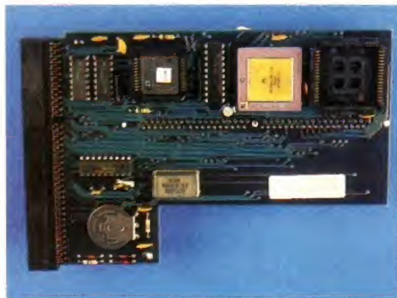
The PC1208 gives you more Fast memory and an FPU running at up to 50MHz.
